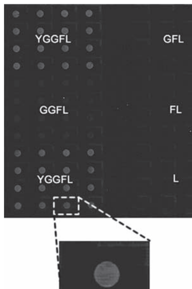
Fig. 11.3 Evidence for the site-selective synthesis of short peptide segments on a microelectrode array having 1028 microelectrodes \text{cm}^{-2}
