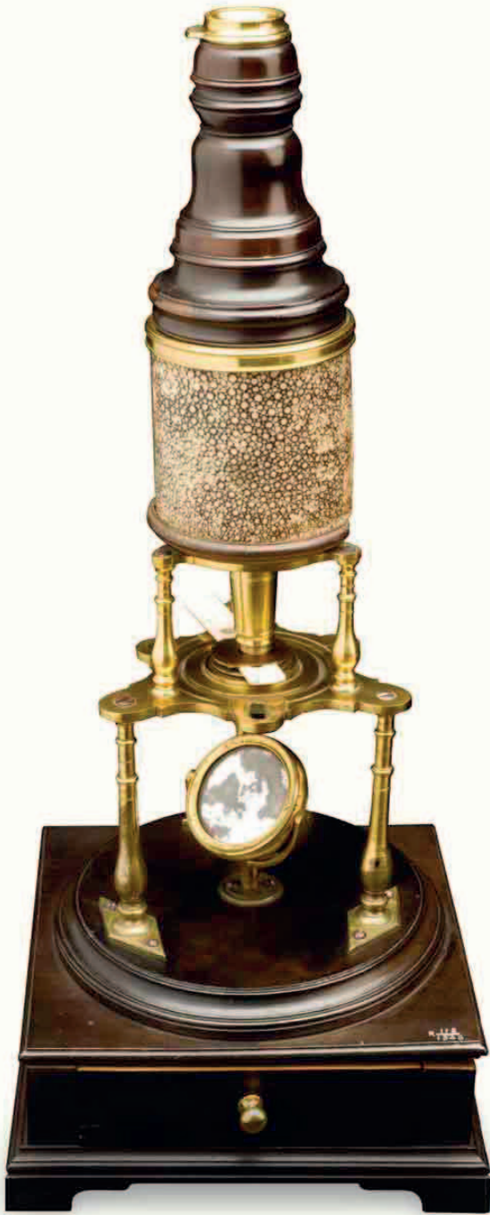
CULPEPER COMPOUND MODEL (1738) British instrument-maker Edward Culpeper's microscope used a concave mirror to illuminate samples. With interchangeable lenses, it could magnify up to x200.
