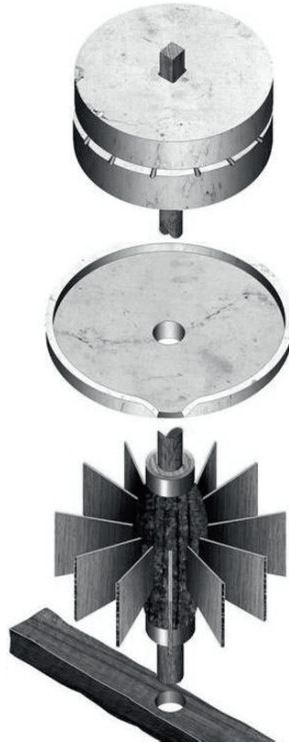
Fig. 6.1 Virtual reconstruction of a vertical axis mill.
