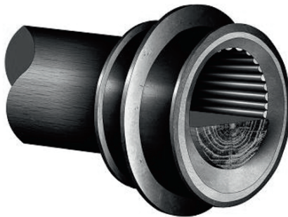
Fig. 10.19 Virtual reconstruction of a Celtic roller bearing.
