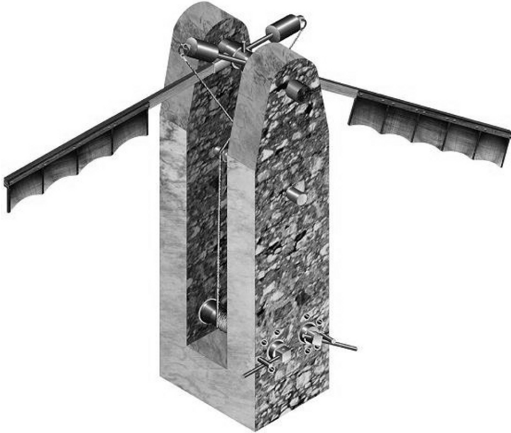
Fig. 11.3 Authors' virtual reconstruction of a Roman rod telegraph.
