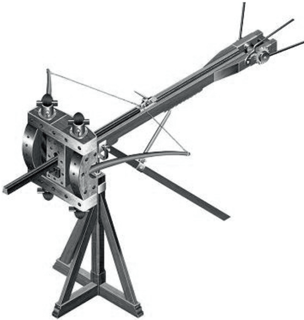
Fig. 12.6 Virtual reconstruction of a Roman catapult with torsion motor.
