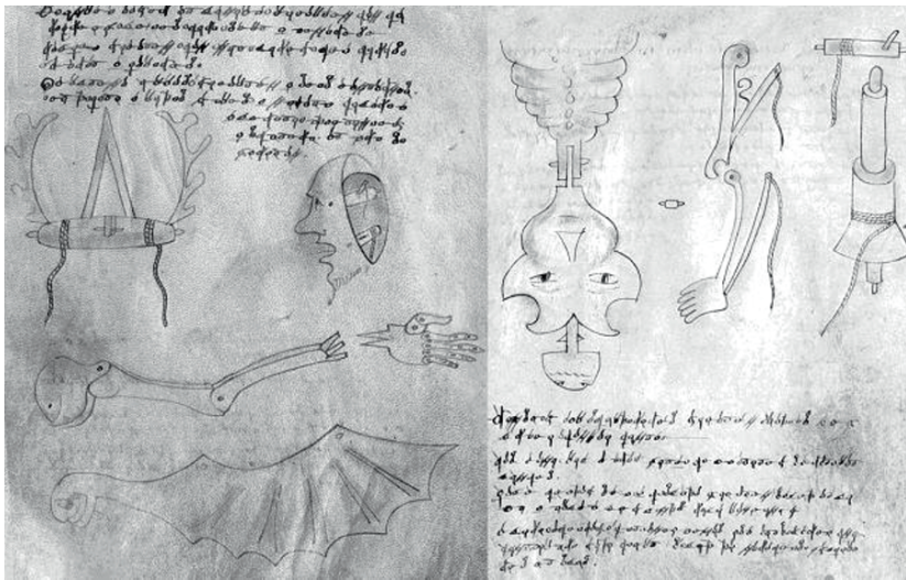
Fig. 15.16 Joints of Fontana's automata.
