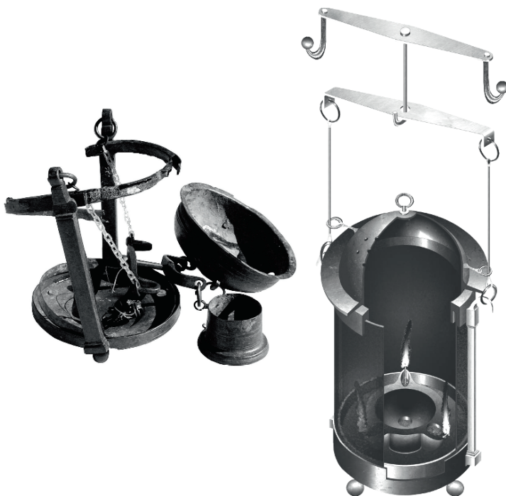
Fig. 14.4 Wind lantern found at Herculaneum and virtual reconstruction.
