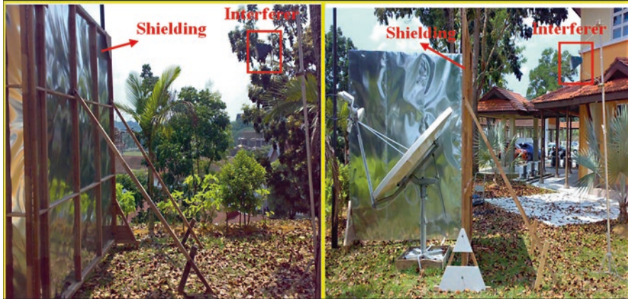
Fig. 4.9 Zinc sheet used in the FSS unit shielding experiment
