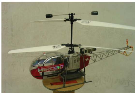
Fig. 1. Micro RC helicopter with the coaxial contra-rotating rotors
