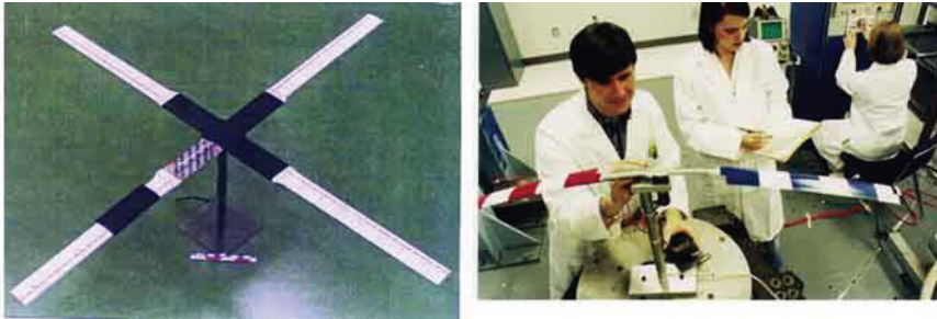
Fig. 14. Solid State Adaptive Rotor with Root Torque-Plate Actuator 38,39
