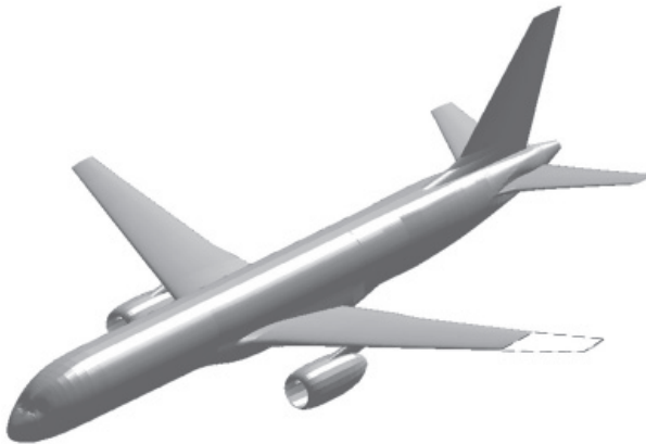
Fig. 2. Left Wing Damaged Generic Transport Model
