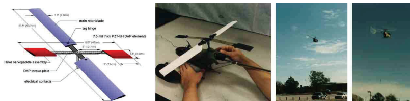
Fig. 15. Gamara, The First Rotary-Wing UAV to Fly with Adaptive Materials for All Flight Control. 39
