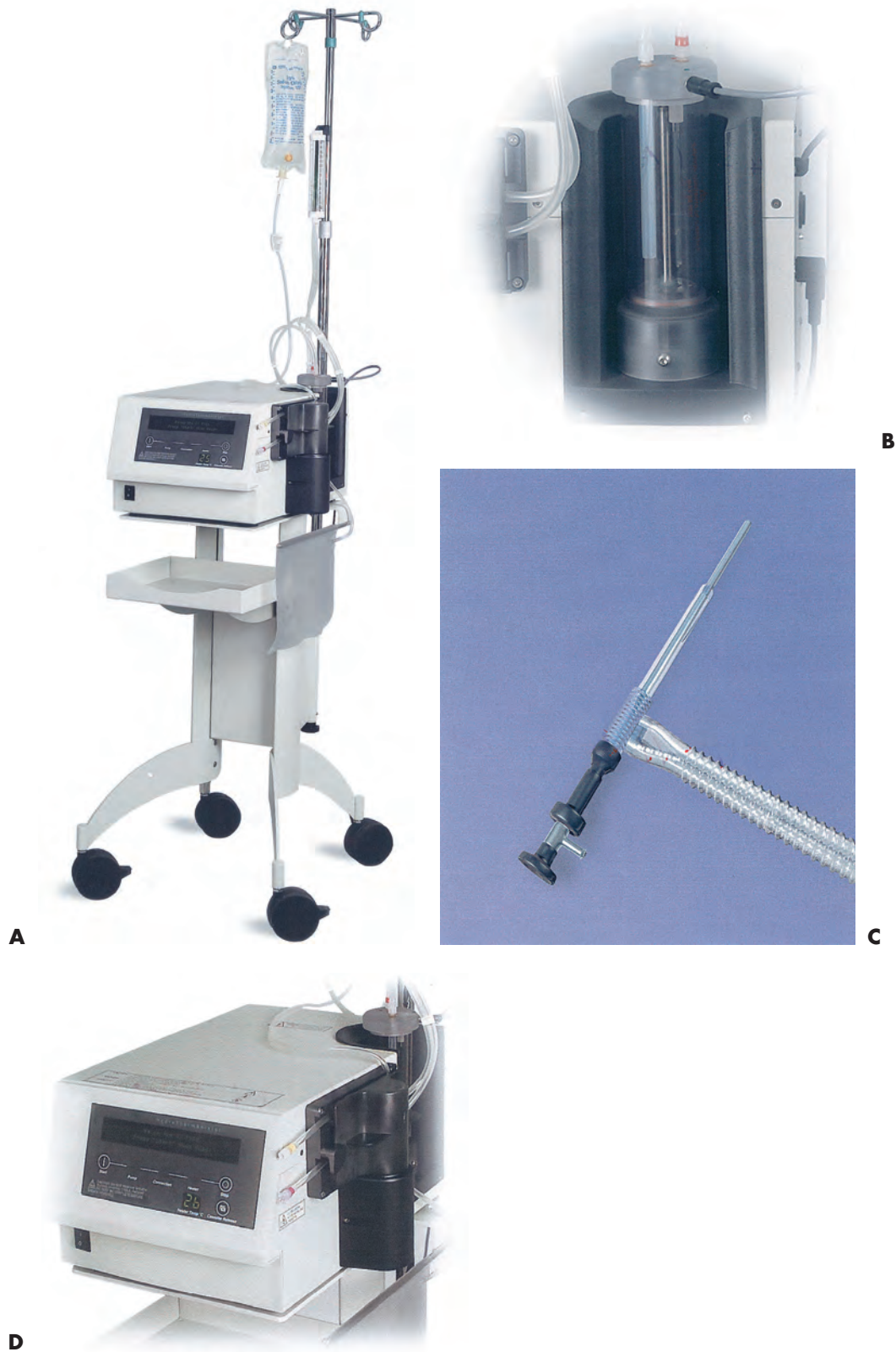
FIGURE 28.22 A: The Hydro ThermAblator (HTA) control unit with reservoir bag of normal saline flowing into the heating unit. B: Magnified view of the outside-the-uterus heating unit. C: The hysteroscope and sheath that deliver the hot saline into the uterus under direct vision. D: The control unit measures intrauterine fluid, pressure, and temperature. (From Baggish MS, Valle RF, Guedj H. Hysteroscopy: Visual Perspectives of Uterine Anatomy, Physiology and Pathology . 3rd ed. Philadelphia: Lippincott Williams & Wilkins; 2007.)
