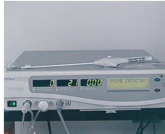
FIGURE 28.18 This cutaway illustration of the uterus shows a fully inflated balloon in place. A: The in situ heating coil is shown together with thermistors and pressure transducers. B: The Gynecare ThermoChoice II intrauterine balloon is shown here with its control unit. C: Magnified view of control unit panel of the control unit. Pressure is read out on the left, temperature within the uterine cavity is indicated in the center, and elapsed time on the far right panel. (From Baggish MS, Valle RF, Guedj H. Hysteroscopy: Visual Perspectives of Uterine Anatomy, Physiology and Pathology . 3rd ed. Philadelphia: Lippincott Williams & Wilkins; 2007.)
