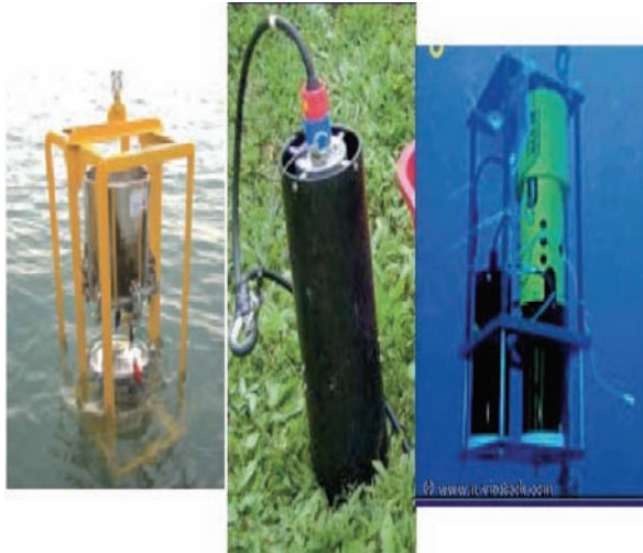
Fig. 1 (Chapter 20). Samples of currently available deployable systems that can be used in situ to sense conditions associated with potential CHAB events. 1). Flow Cam system from Fluid Imaging Technologies can identify cell type in situ. 2). Fluoroprobe system can identify water column phytoplankton based on a combination of 6 different fluorescence signatures. 3). NAS nutrient analyzer can detect in situ biogeochemical shifts that can be linked to pending CHAB events. (See page 477).
