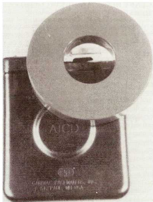
FIG. 22-6. Correct magnet placement to deactivate second-generation ICD. (Reproduced with permission from Chapman PD, Veseth-Rogers JL, Duquette SE: The implantable defibrillator and the emergency physician. Ann Emerg Med 18:579, 1989.)
