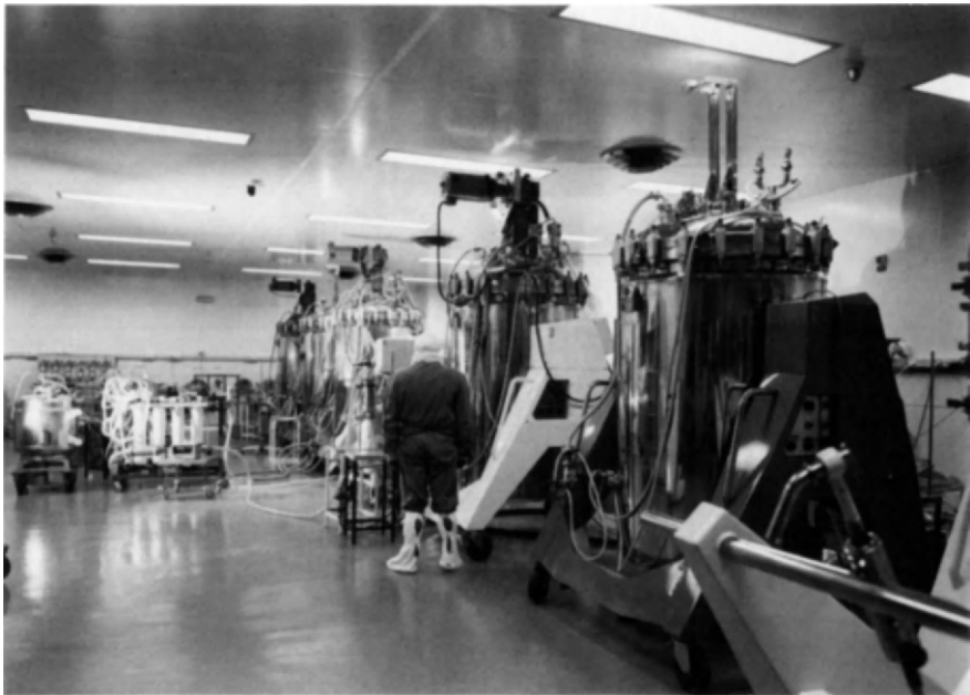
Fig. 5. Cytogenerator for mass culture of VERO cell.
