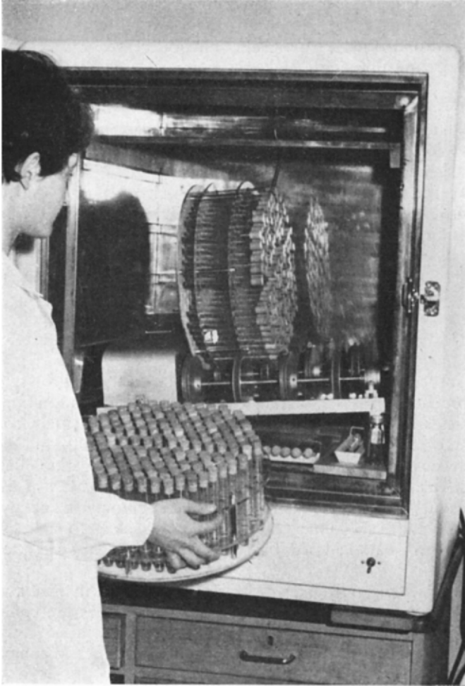
FIG. 5.1. Roller-drum apparatus ( Matburn Ltd. ) in a water-jacketed, 37°C, incubator ( Laboratory Thermal Equipment Ltd. ). (Photo— W. Topp. )
