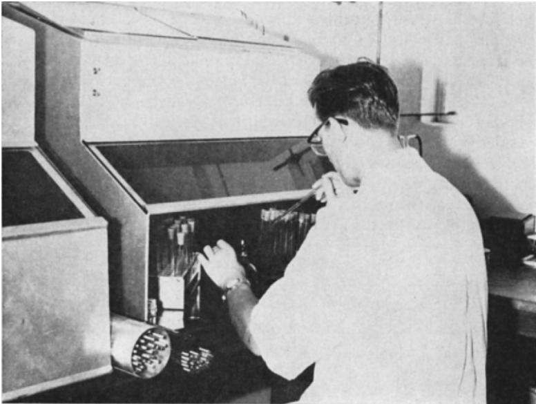
FIG. 1.1. Working with tissue cultures under a hood which can be sterilised by ultra-violet light when not in use. (Photo—L. E. Hewitt.)
