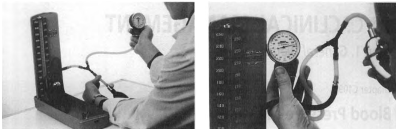
Figure C103.1 Aneroid instrument being tested by inserting a Y-tube connector or stopcock to create a communicating system with one pressure source, allowing simultaneous pressure application to both instruments. (Courtesy of Shared Care Research and Education Consulting, Inc., Milwaukee, WI.)
