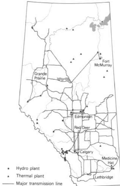
Figure 7-8 Alberta's electric power transmission grid and locations of electricity generating stations in 1981. Source: Government of Alberta.
