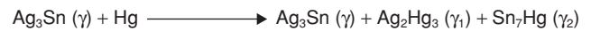
Figure 9.3 The setting reaction for traditional dental amalgam. There will be an amount of \gamma phase remaining in the final material, as not all of each particle is dissolved into the mercury. The \gamma_2 phase has adverse effects on the properties of the material.
