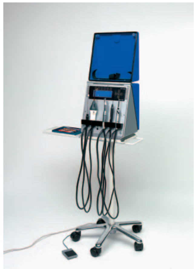
Figure 15.4 Portable dental equipment (Mini-dent). Reproduced by kind permission of J&S Davis.
