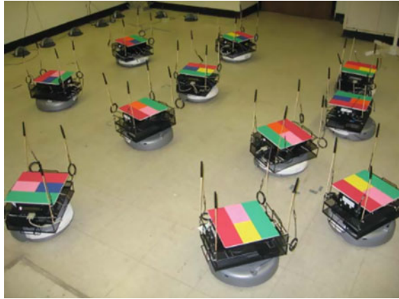
Fig. 5.15 MiNT-m prototype with 12 nodes and charging stations (top left corner) (De et al. 2006)
