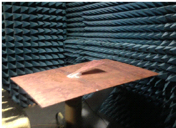
Figure 8.26 A set with the model of an antenna placed on the faces of a regular pyramid.
