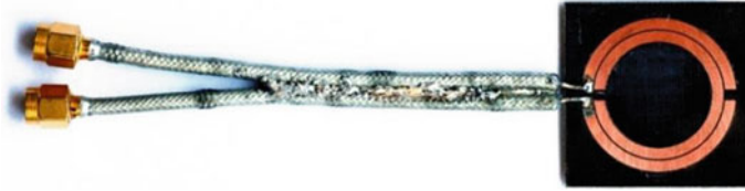
Fig. 3.4 SRR antenna input impedance measurement assembly. Reprinted with permission from [3]
