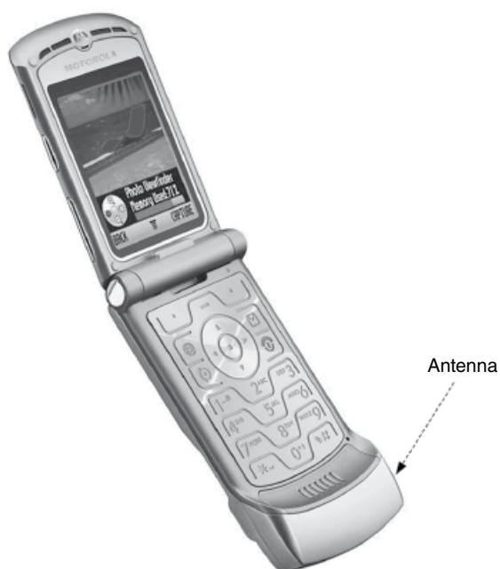
Figure 1.6 Bottom internal monopole antenna on a Motorola Razr V3 (2004). (Source: Reproduced with permission of Motorola.)
