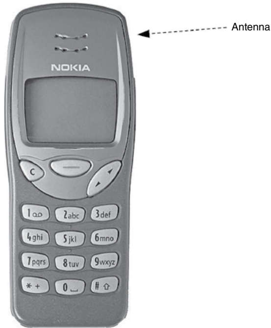
Figure 1.5 Nokia, Inc. Internal antenna on a Nokia 3210 (1999). ( Source: Reproduced with permission of Nokia.)
