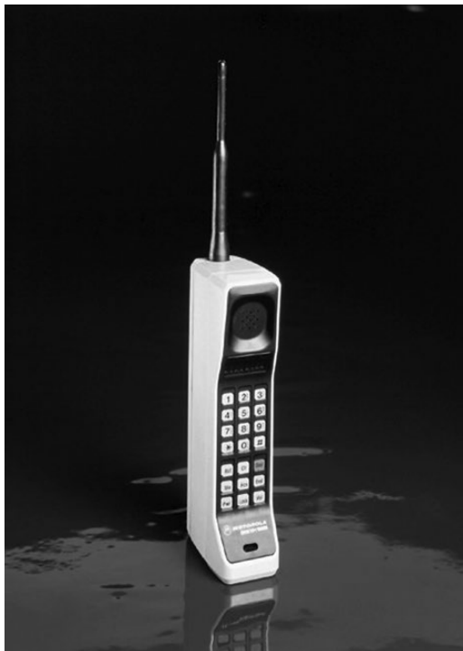
Figure 1.1 Sleeve dipole antenna on a Motorola DynaTAC 8000X (1983). ( Source: Reproduced with permission of Motorola.)
