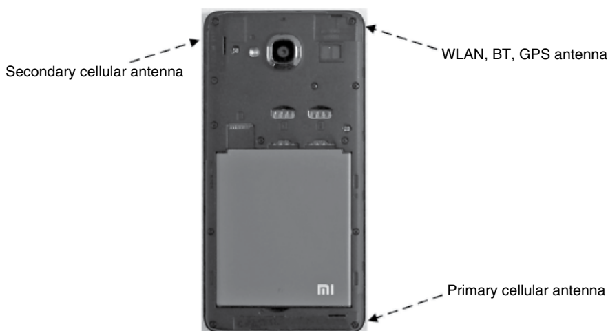
Figure 4.96 Hongmi 2A with back cover detached. (Source: Reproduced with permission of Xiaomi, Inc.)
