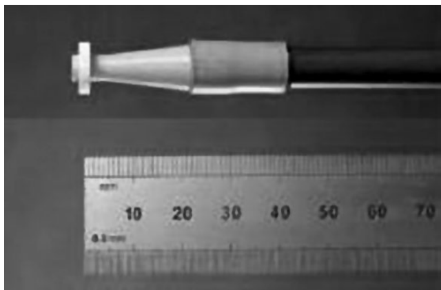
Figure 6.27 Probe for T-coil measurements. (Source: IndexSAR Ltd.)
