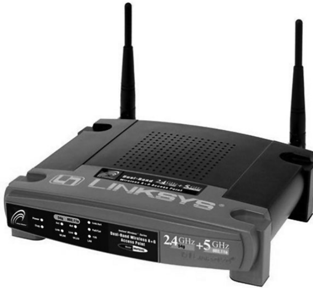
Figure 1.2 Sleeve dipole antennas on a wireless LAN access point. Linksys WAP55AG. (Source: Cisco, Inc.)
