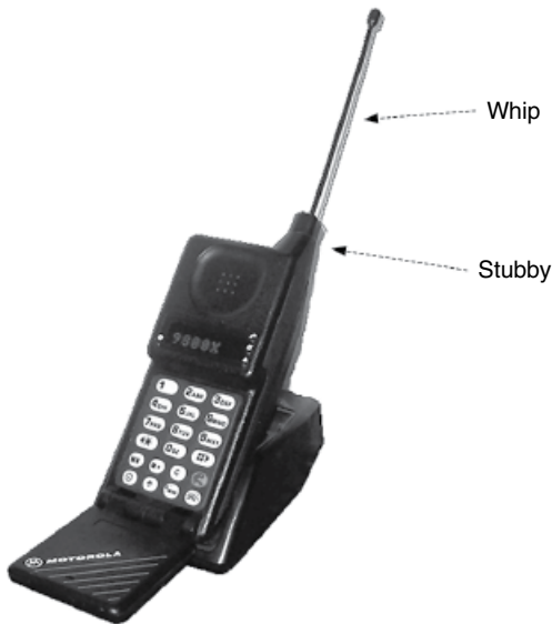
Figure 1.3 Whip antenna on a Motorola MicroTAC 9800X (1989). (Source: Reproduced with permission of Motorola.)
