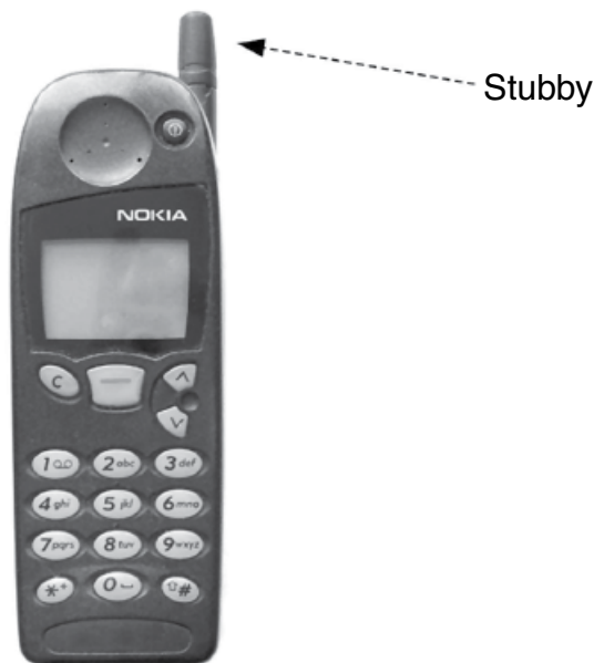
Figure 1.4 Nokia, Inc. Stubby antenna on a Nokia 5110 (1998). (Source: Reproduced with permission of Nokia.)
