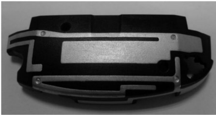
Figure 4.35 Antenna made by DS-MID technology. (Source: Reproduced with permission of Shanghai Amphenol Airwave.)
