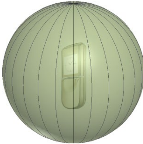
Figure 5.26 Measurement 3D sphere of a Satimo chamber (15° step).
