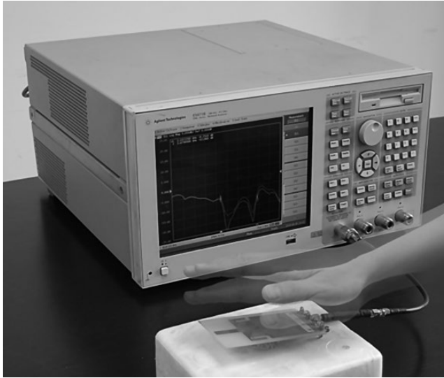
Figure 5.6 Use hand to quickly check an antenna's performance.
