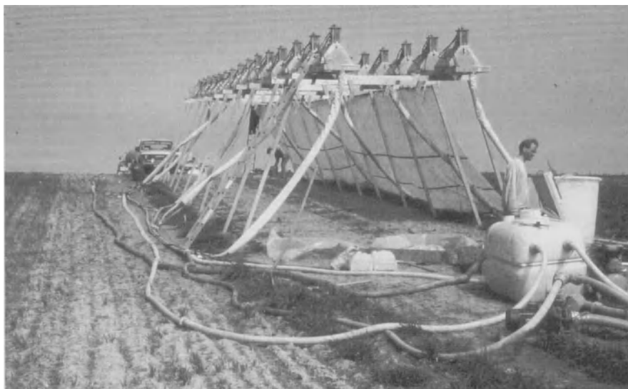
Fig. 6.4. Plot rainfall simulation used for experimental investigation of soil erosion and sediment-bound heavy metal transport
