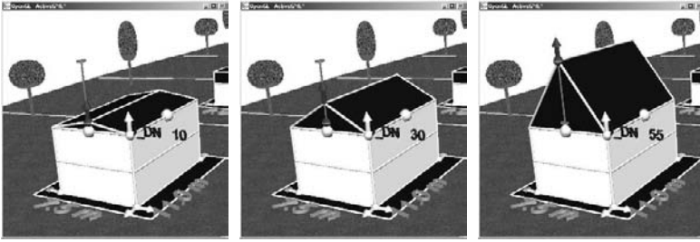
Fig. 23.7. Interactively changing of height of the roof within the given constraints of the zoning map. The roof pitch varies from 10 to max. degree in this example.
