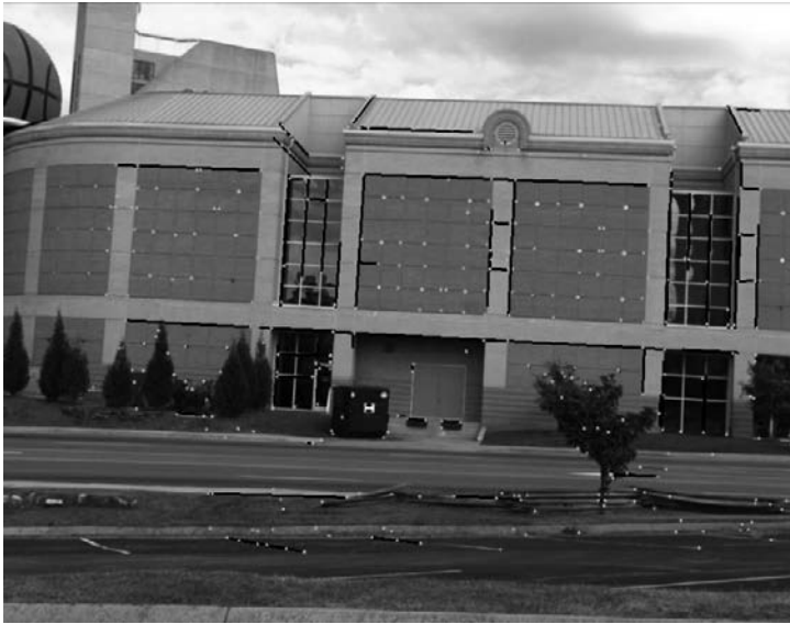
Fig. 14.1. Feature extraction result, reliable points (dot), matched edges (finite line)
