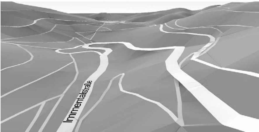
Fig. 8.12. Certain mountain roads have been integrated into the terrain and flattened. Major roads have a higher priority and were flattened more than smaller forest tracks.
