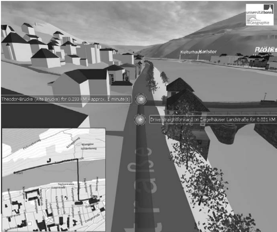
Fig. 8.9. Display of a route integrated into a 3D city model with corrected road surface. The route goes right onto the bridge.
