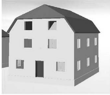
Fig. 6.5. Geometrical Representation of a building in CityGML LOD 3 (CityGML Dataset, Four Buildings in LOD 3)
