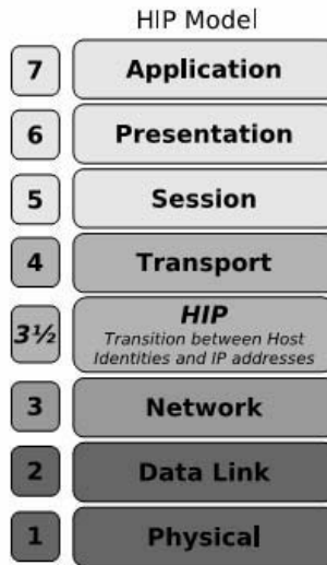
Figure 1.12. Host Identity Protocol in ISO layers [HIP]
