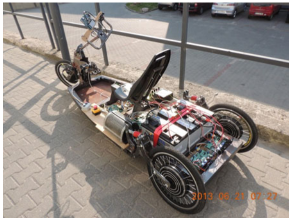
Fig. 2 The view of the vehicle prototype intended for traction tests
