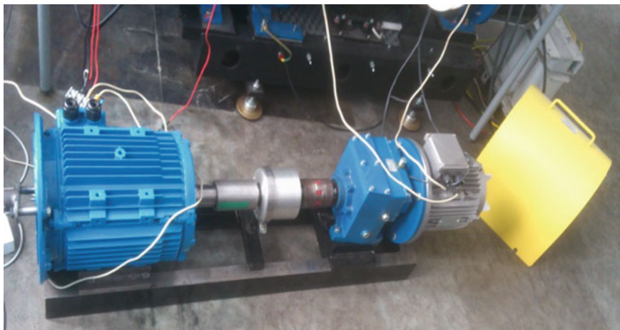
Fig. 18 View of the test rig with the 2 kW generator
