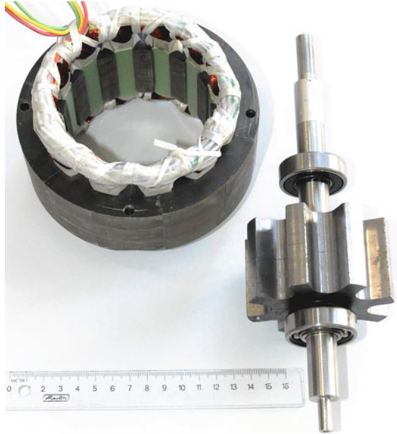
Fig. 3 The stator and rotor of the switched reluctance motor made of soft magnetic composites
