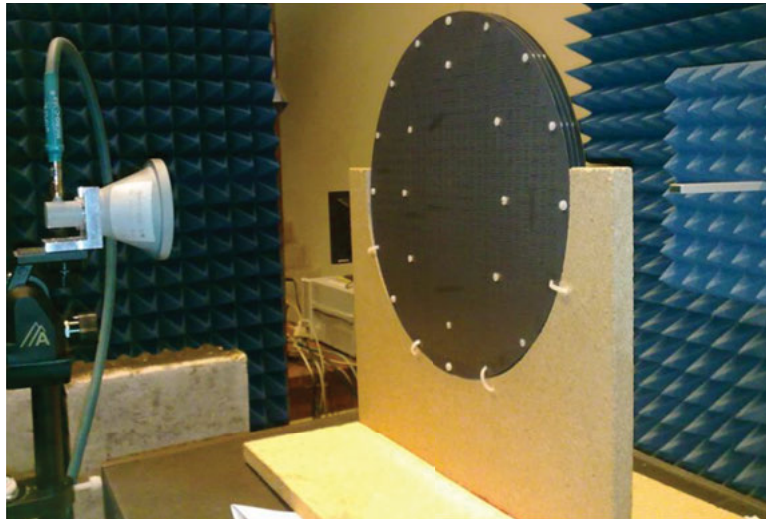
Figure 7.7: Near-field measurement setup of the single-feed quad-beam transmitarray antenna.
