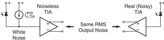
Figure 5.14 Interpretation of the averaged input-referred noise current density.
