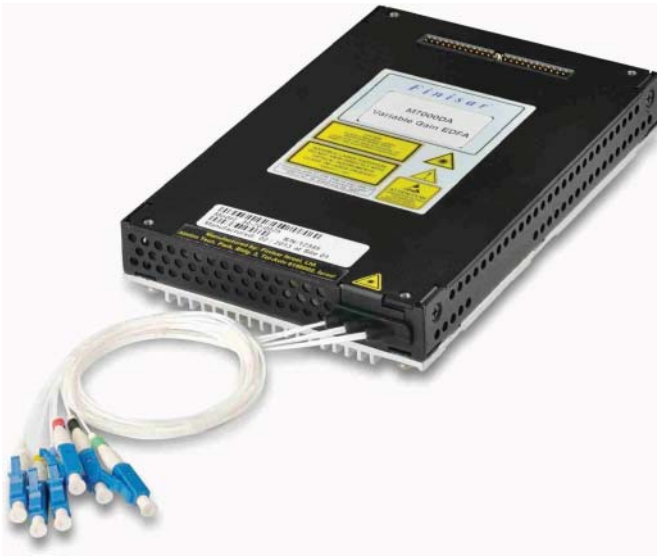
Figure 3.19 A packaged variable-gain two-stage erbium-doped fiber amplifier with single-mode fiber pigtailed for the input, output, and interstage access (15 cm × 10 cm × 1.8 cm). Source: Reprinted by permission from Finisar Corporation.
