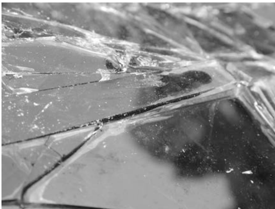
FIG. 5.6 A: The laminated windshield glass fractures into shards. Blood and hair are easily deposited during contact. B: Contact with windshield glass results in linear incised wounds.
