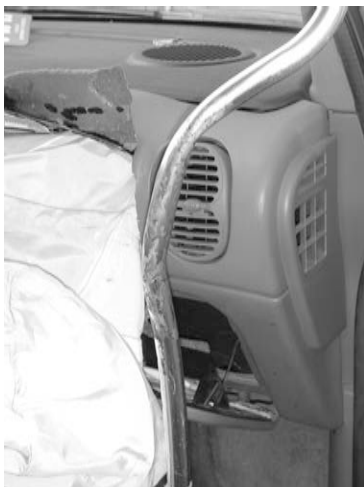
FIG. 5.20 A metal cane was propelled rearward by the deploying passenger air bag into the passenger's right eye (Fig. 5.21).
