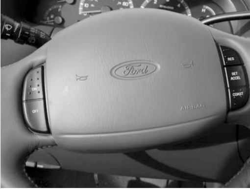
FIG. 5.29 Horn buttons located within the module cover are an invitation for hand and arm injuries if the driver attempts to blow the horn during a frontal impact.
