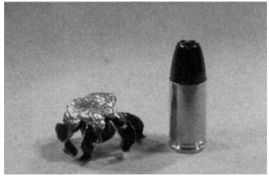
FIG. 4.3 Hollow-point ammunition, like this 9-mm "Black Talon" bullet, has the capacity to significantly increase its surface area upon impact with tissue.
