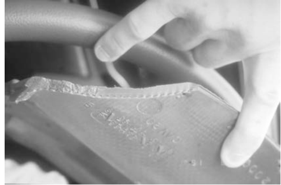
FIG. 5.31 The module cover from a 1991 Ford Taurus was torn by impact with the left side of the restrained driver’s face. This force associated with air-bag deployment and module cover impact resulted in a fatal head injury.
