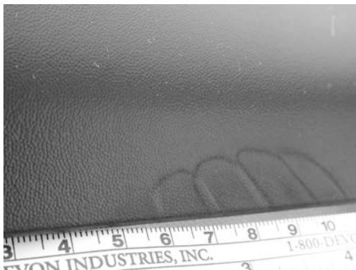
FIG. 5.12 The imprint of a shoe was transferred to the air-bag module cover. The passenger had her foot on the module cover at the moment of deployment (Fig. 5.19).
