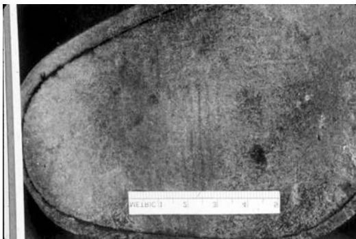
FIG. 5.8 An imprint of the brake or accelerator pedal can be transferred to leather soles. Examination of shoes can assist in the determination of an occupant's role.
