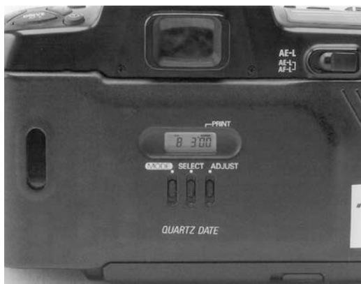
FIG. 17.16 A databack imprints the date, time, or sequence number on the film. This option assists the emergency department photographer in dating the photograph.
