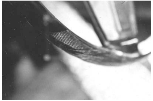
FIG. 5.9 Forceful impact of clothing against vehicle components can impart a fabric transfer. The comparison of the fabric weave from the imprint on the steering wheel assisted in determining which occupant was the driver.
