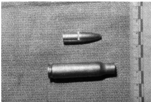
FIG. 4.2 A .308 caliber high-velocity rifle round. By virtue of their speed, high-velocity rounds have the potential to transfer large amounts of energy to body tissue.
