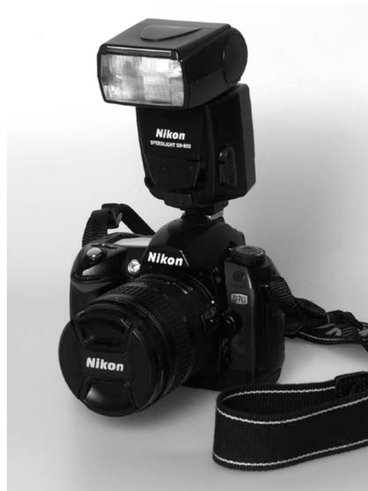
FIG. 17.23 The Nikon D70 produces a near-film-quality photograph with a 6.0 million pixel image.
