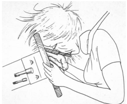
FIG. 5.18 Impact of the deploying module cover with the face can cause serious, even fatal, cranial and cervical spine injuries.
