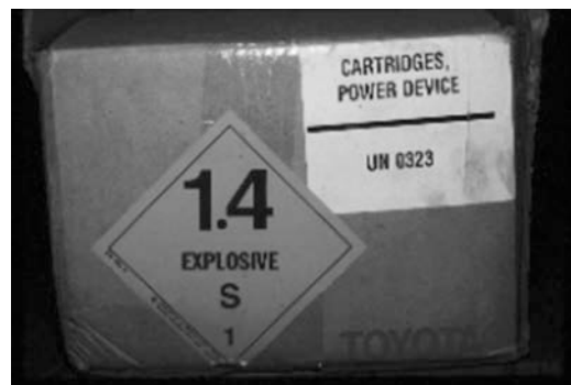
FIG. 5.14 Sodium azide is a toxic explosive material used for nitrogen generation in first-generation air bags. When not completely consumed in the inflation process, sodium azide has caused severe damage to the eyes and respiratory tract.
