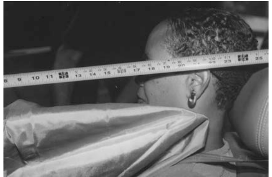
FIG. 5.27 Untethered air bags can extend rearward more than 20 in. and inflict facial injuries in properly restrained drivers and passengers. The untethered air bag in this 1989 Acura struck the driver's left eye, resulting in a lid laceration and ruptured globe.
