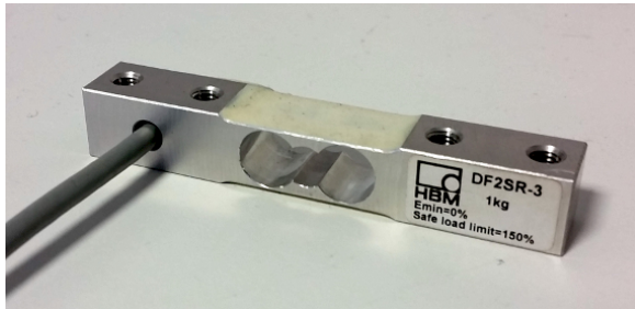
Figure 1.26. Photograph of the load cell DF2SR-3 from HBM. The strain gages are glued to a spring, whose deformation is translated into a differential voltage
