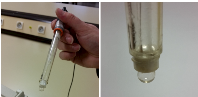
Figure 1.6. Photographs of the Sentek P14/S7 electrode for pH measurements
