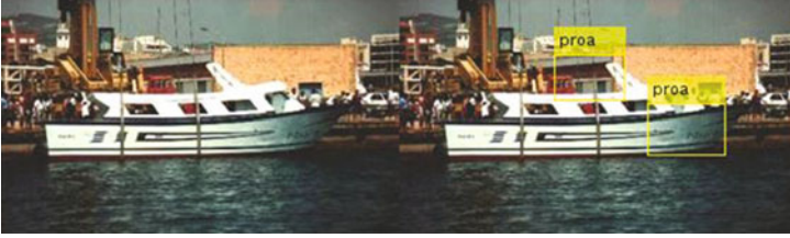
Fig. 3. Identification of vessel bow through HOG process
