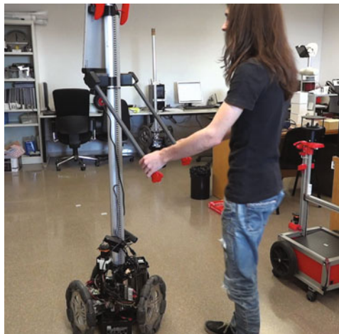
Fig. 3. User activating the walker mode of the APR
