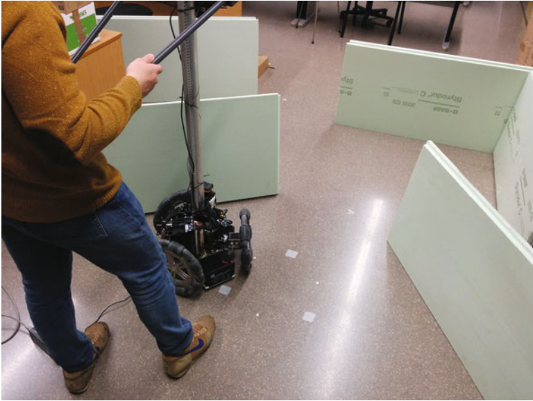
Fig. 5. User controlling the APR in walker-helper mode passing through obstacles
