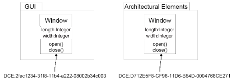
Figure 2. Unique identification of elements using UUID
