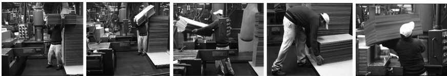
Fig. 1 Feeding task: take from the pallet a group of cardboard and place in the feeder mechanism repeated times until the material stocked is finished
