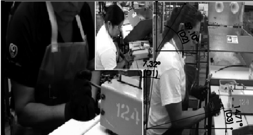
Fig. 3 Wrong posture in the assembly of spark plug wires
