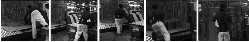
Fig. 2 Downloading task: take a packet of cardboard from the rolled conveyor and put over pallet repeated times until the pallet is completed
