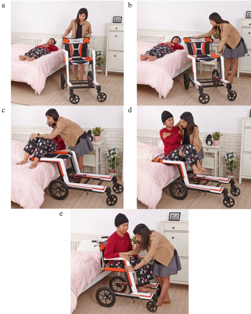
Fig. 5 The process of transfer aid: a the transfer aid is moved to parallel side of the bed; b the armrests are then lowered, and handles and seat back folded up; c the seat is unlocked and slid onto the bed; d the care demander pivots from supine to sitting at the edge of bed; e the care demander along with the seat are slid back the transfer aid, and the armrests, handles, and the seat back are pulled back to their original positions
