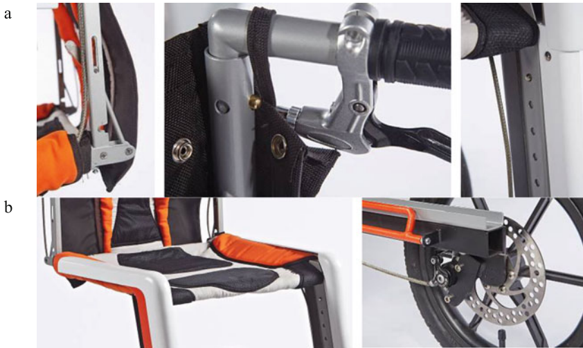
Fig. 4 Detail design of transfer aid a a foldable seat back, two foldable handles and two adjustable armrests b a movable seat and wheel
