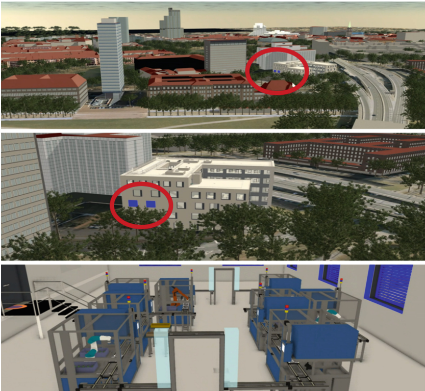
Fig. 4. Consistent large-scale environment model from CityGML and BIM with detailed robot simulation [8]
