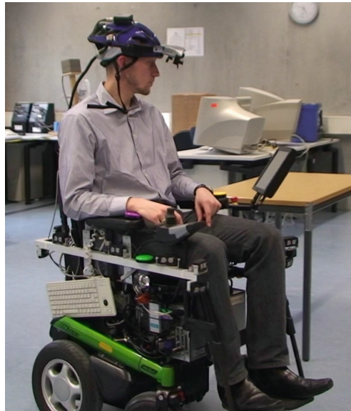
Fig. 1. Wheelchair prototype with head-mounted eye tracking system and real-time control system providing multiple assistance behaviours [4].
