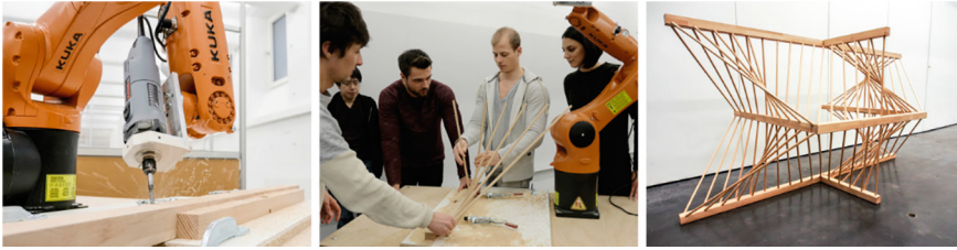
Fig. 1. Collaborative fabrication: robotic milling (1), manual assembly (2), assembled design object (3)
