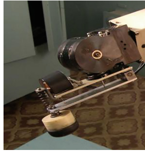
Fig. 6. Biomechatronic module with one-component force induction sensor
