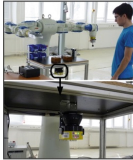
Fig. 2. Location of 2D laser scanner on the work desk of robot within cooperative workplace
