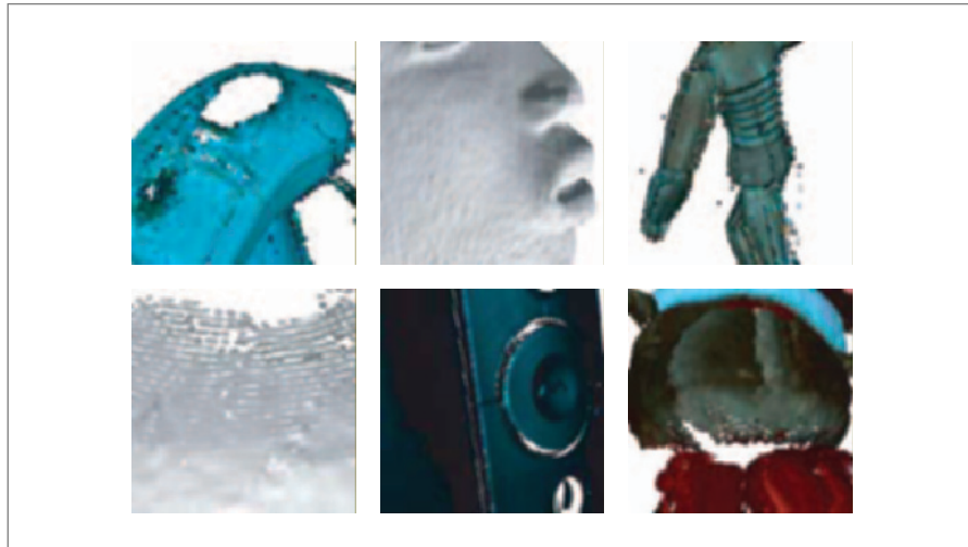
Figure 5.1: Typical artifacts of raw scanner data. Top row: Holes due to sensor restrictions, noise, outliers. Bottom row: Low sampling density due to gracing sensor views, low sampling density at delicate surface details, and holes due to critical reflectance properties.
