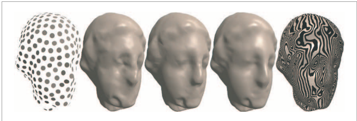
Figure 4.54: Right: The Igea model uniformly sampled by 600 points is refined to 150,000 points with various techniques. Then, from left to right: The butterfly (after a meshing step), a dyadic refinement of point clouds [GBP04], and the \sqrt{3} -like refinement. The last picture is rendered with reflexion lines showing normal and curvature variations.
