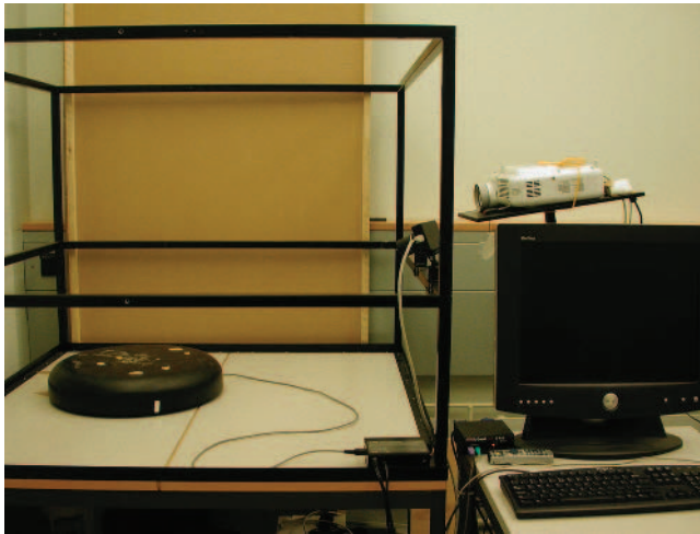
Figure 3.9: System overview: turntable, camera, projector, and control computer (from left to right ).
