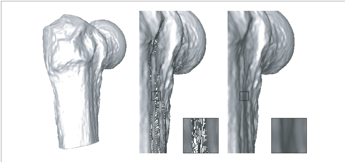
Figure 6.17: Local affine approximations to the projective mapping can cause holes for extreme viewing angles ( center ). These holes can be closed either by an affine approximation that correctly maps the outer splat contour or by perspective-correct per-pixel ray casting ( right ).
