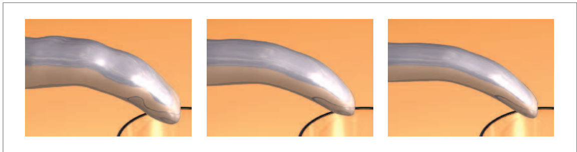
Figure 7.24: The effect of the different potential functions on the surface: (a) guiding potential, (b) smoothing potential, and (c) attracting potential.
