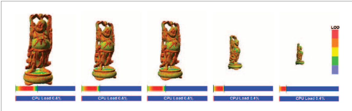
Figure 6.44: Continuous detail levels of a Buddha generated in vertex programs on the GPU. The colors denote the LOD level used and the bars describe the selected amount of points selected for the GPU. CPU load is always below 1%.
