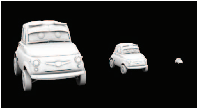
Figure 8.54: Direct rendering of the Fiat Topolino ambient occlusion brick map at three different sizes.
