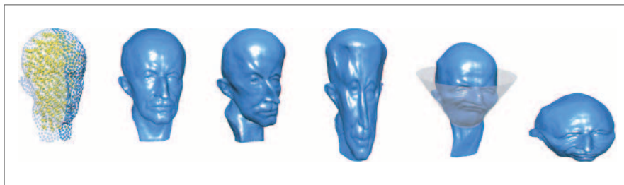
Figure 7.7: The model presented in this chapter represents both the physical volume elements (phyxels in yellow) as well as the surface elements (surfels in blue) as point samples. It allows the simulation of elastic, plastic, melting, and solidifying objects (from left to right ).
