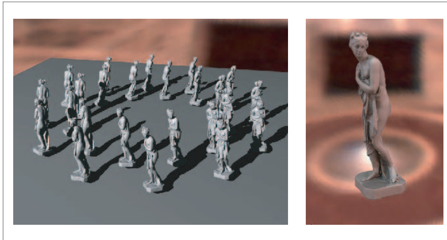
Figure 6.36: Interactive ray tracing. (a) A scene consisting of 24 Iphigenias with a total of 24 million points with Phong shading and shadows rendered at two frames per second at 640 \times 480 image resolution. (b) One Iphigenia rendered with precomputed global illumination at four frames per second for a resolution of 400 \times 600 pixels. Images taken from Wald and Seidel [WS05].
