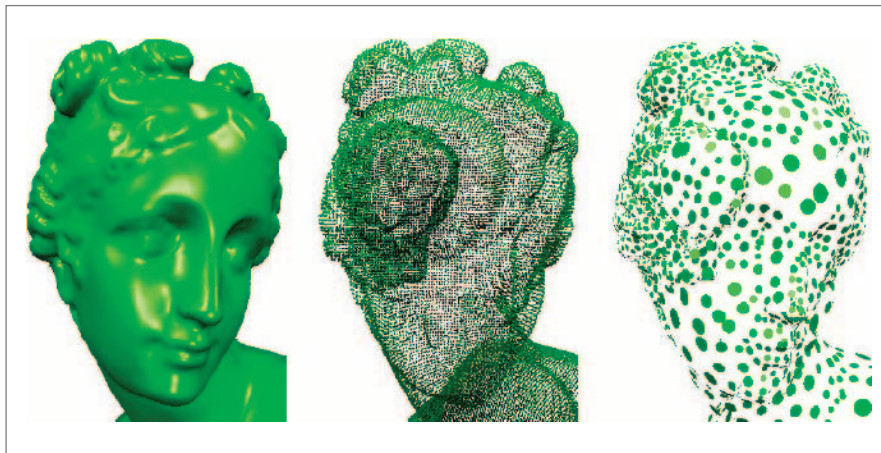
Figure 4.21: The original point model ( left and middle , 352,000 points) is decimated to 30,000 circular surface splats ( right ).
