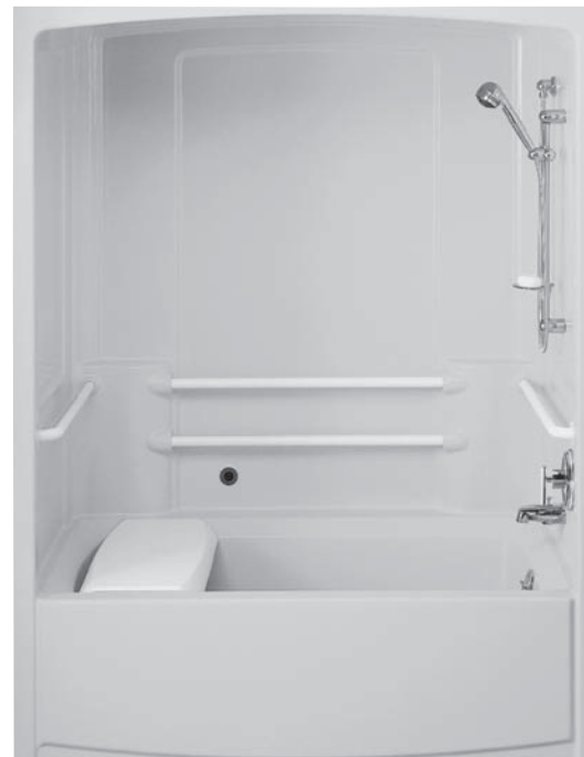
Figure 6-18b Prefabricated bathtub/shower module for wheelchair transfer with a seat, multiple grab bars, handheld shower spray, and controls mounted near the entry side of head wall. Many users prefer the addition of a vertical grab bar at the control side of tub. Note: Showers are generally the best option for wheelchair users.
