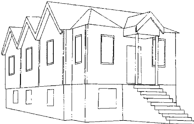
2-14. Sketch of a chattel house, Barbados. Although not shown in this drawing, the rear sections are sometimes a bit wider than the original front section in order to provide better ventilation. Each section can be disassembled quickly for moving to a new site. Most chattel houses do not have basements. (drawing by Amy Rock).
