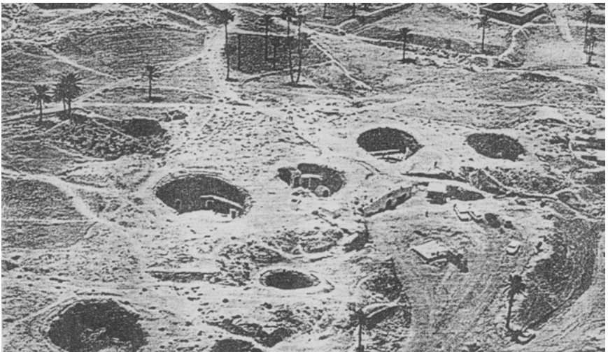
7-11. An aerial view of open, sunken courtyards in the Matmata plateau. The openings to several caves can be seen appearing obliquely in the courtyards (from a portion of a photograph in Golany 1988, 49. Reprinted with permission of the University of Delaware Press).
