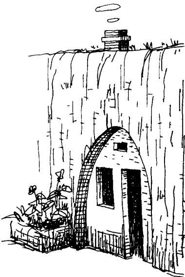
7-8. Typical vaulted facade of a loess cave located along a road cut or a vertical cliff. Note the chimney protruding out of the upper ground surface (from Golany 1992, 104. Reprinted with permission of the University of Hawaii Press).
