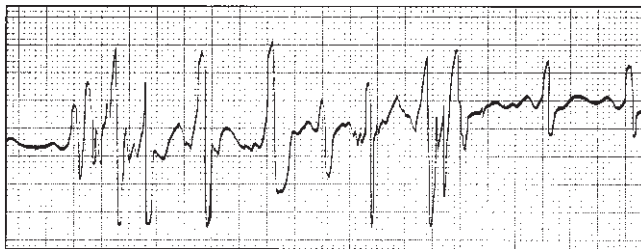
Fig. 2.16 Poor electrode connection (reproduced by kind permission of Medicotest, manufacturer of 'blue sensor electrodes')
