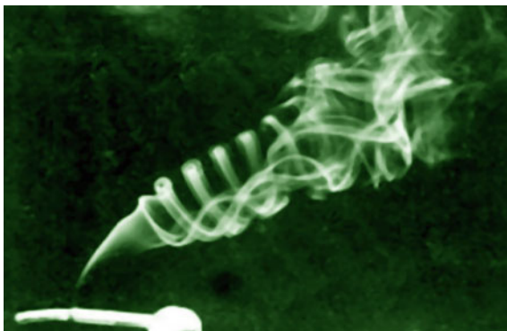
Fig. 6.6 Humorous picture of self-organized perturbation of cigarette smoke oscillations showing general impact of Bernoulli–Kelvin–Helmholtz instabilities proficient on any scale
