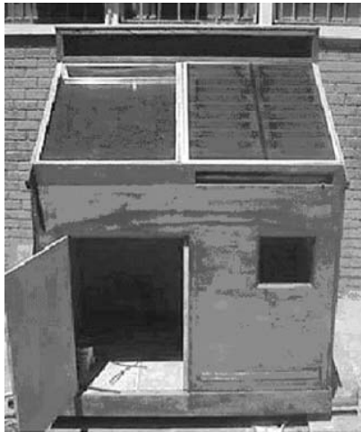
Figure 8. A solar test cell to study the performance of energy roofs with embedded PV panels. The design is such as to run the PV powered roof under the PV + thermal concept. The south wall painted greenish functions under the passive solar concept as explained below.
