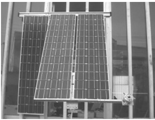
Figure 2a. PV-module from monocrystalline silicon mounted on the south wall of the R.E.S. Lab. of the T.E.I. Patra. This PV system powers house appliances which simulate a household, as installed within the space of the laboratory.
