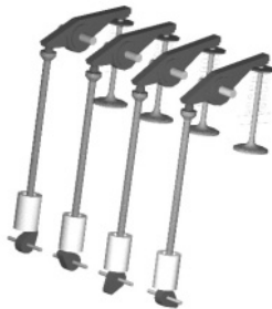
Figure 5. General view of a line valve trains for a four cylinder engine
