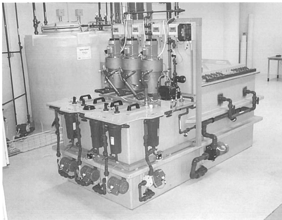
Fig. 14.17 Copper recovery units (MECER) integrated in the production of printed circuit boards. This photograph shows the solvent extraction unit.
