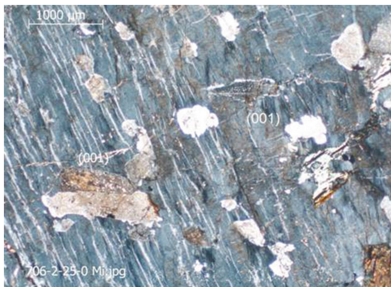
Fig. 3.34 (+). Random distribution of isometric crystals of plagioclase enclosed in K-feldspar Section is along (010)
