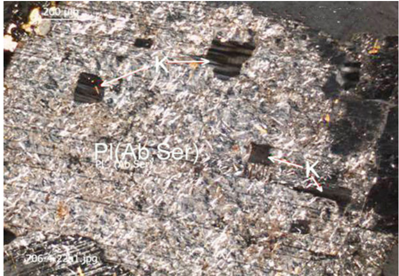
Fig. 1.65 (+). Plagioclase is sericitized and albitized with unchanged remnants of antiperthitic K-feldspar (with very dark gray interference color). Jiling granite
