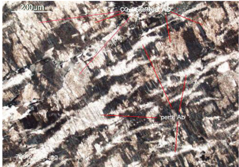
Fig. 1.70 (+). Section is roughly //axis b . K-feldspar is subjected to co-oriented albitization in slices or pile form, accompanied with hydrohematite ( brown and dirtier )
