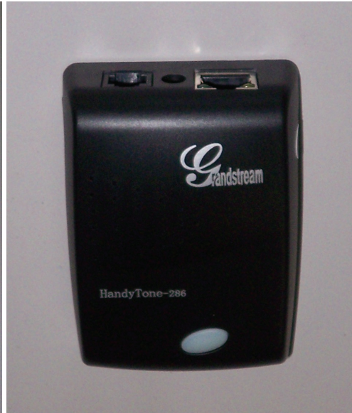
Photo 3. Grandstream HT286 as VoIP Adaptor
