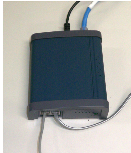
Photo 4. Sipura SPA1000 as VoIP gateway
