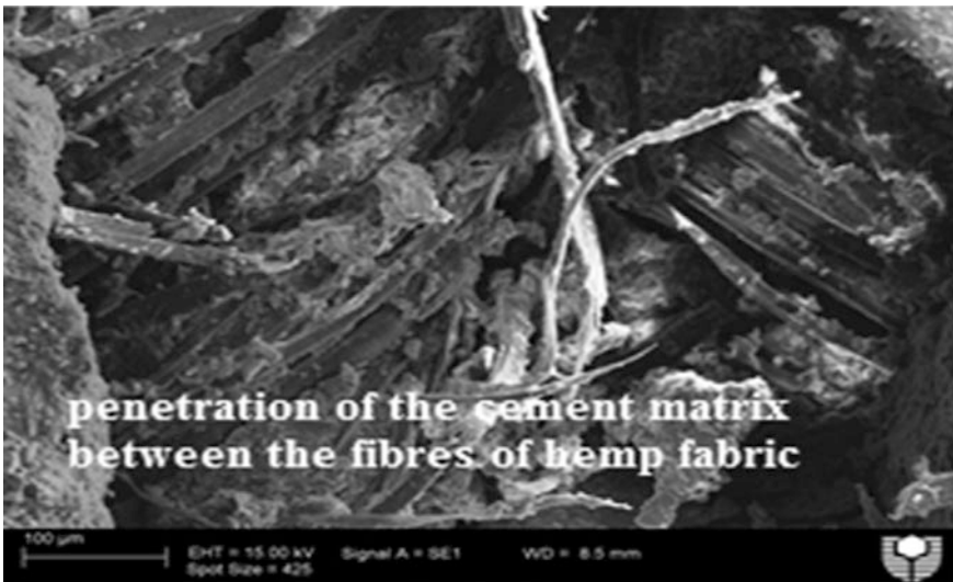
Fig. 3.5 Penetration of the cement matrix in between the reinforced fibres of hemp fabric [1]
