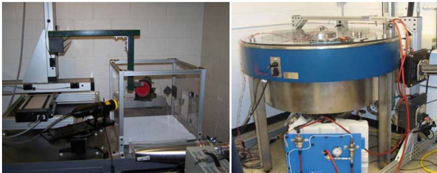
Fig. 15.8 Spray quality measurements equipment. Left PDPA. Right Patternator
