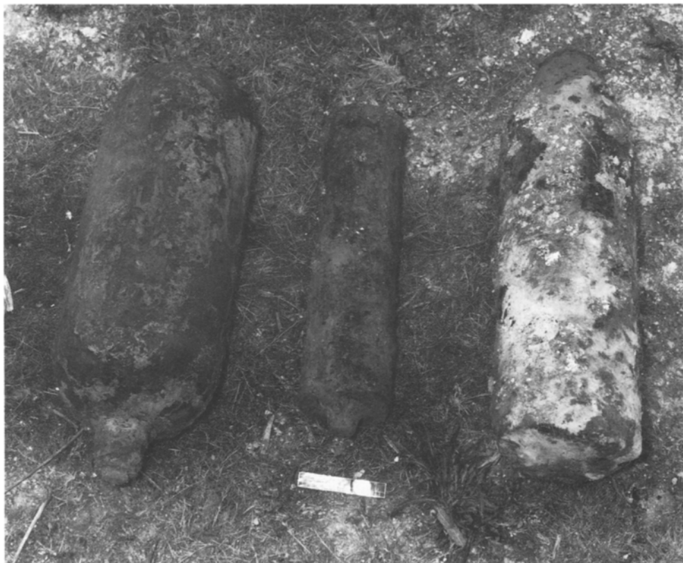
Fig. 1.31 From left to right: a Livens container (phosgene), a 4" Stokes (Mortar Bomb (chloropicrin) and a 6" shell (mustard gas), found buried at Bramley in 1987 (reproduced with permission of the Chemical Defence Establishment, Porton Down). They all exhibit an advanced state of corrosion.
