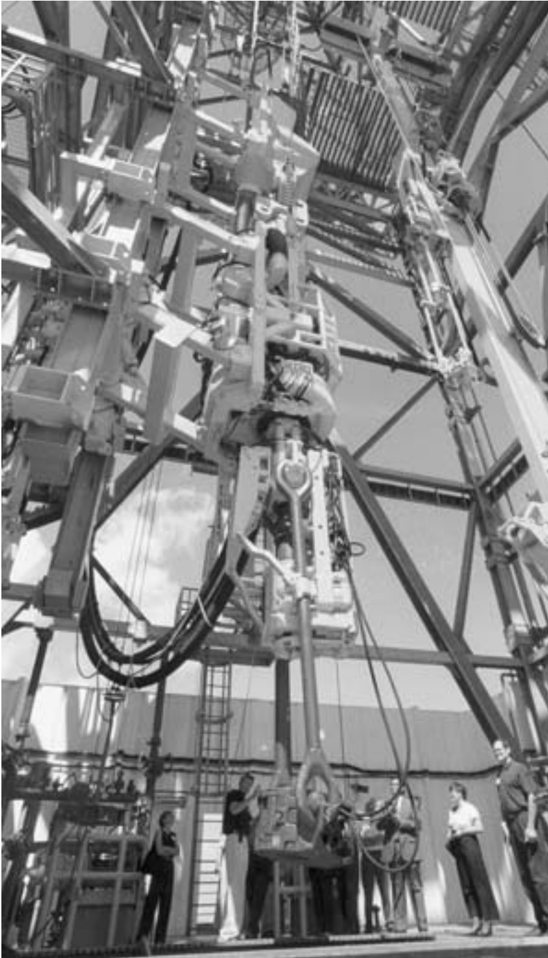
This offshore drilling unit is currently operating in the Gulf of Mexico. The semisubmersible unit, owned by ENSCO, a science, engineering, and technology company, can drill to a depth of 30,000 feet (9,000 meters) and operate in waters up to 8,000 feet (2,400 meters).
