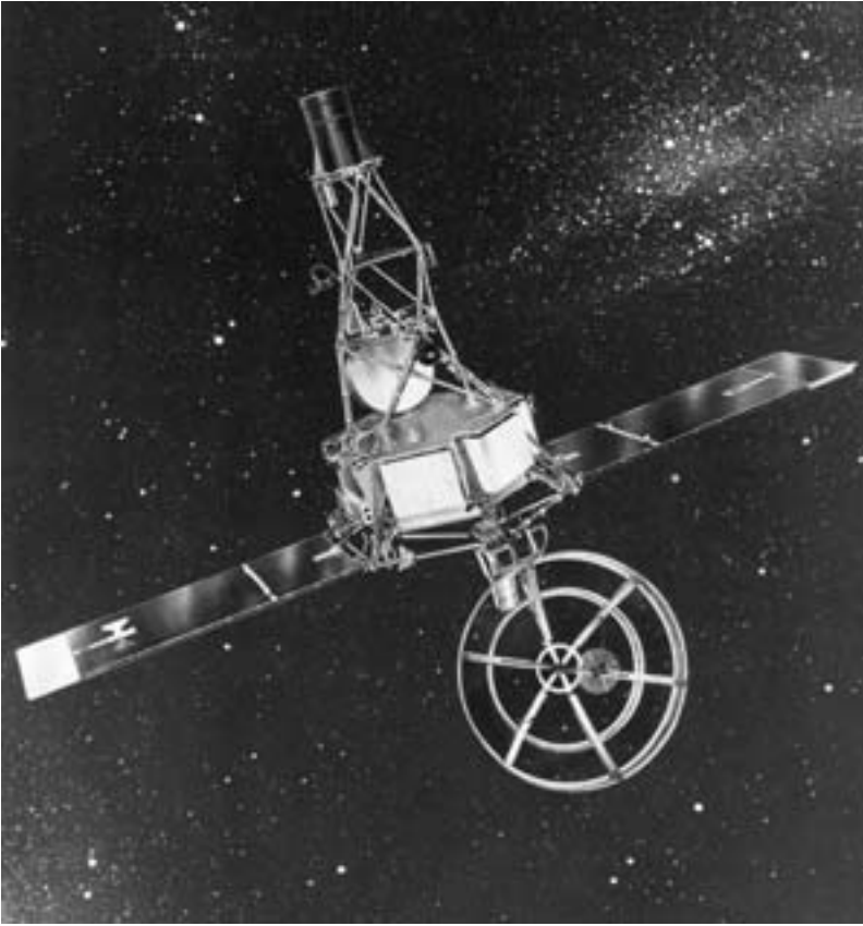
The Mariner 2 spacecraft launched in 1962 speeds toward Venus, improperly unfolding its solar panels in the process. The glitch didn't keep Mariner 2 from becoming the first spacecraft to fly by a planet or from sending back valuable information on the temperature of the clouds and surface of Venus.
