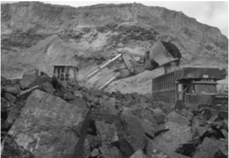
Coal production may see even more of an increase in the next decade as tensions in the Middle East threaten our ability to obtain oil from overseas. In this open pit coal mine in Illinois, large chunks of coal are dug out from more than 70 feet (21 meters) below the earth's surface.
