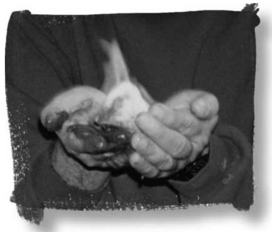
Figure 4. Burning the methane that is released as a gas hydrate sample decomposes. Hands belong to Robert Collier (College of Oceanic and Atmospheric Science, Oregon State University). Picture taken by one of the authors (M. Torres).
