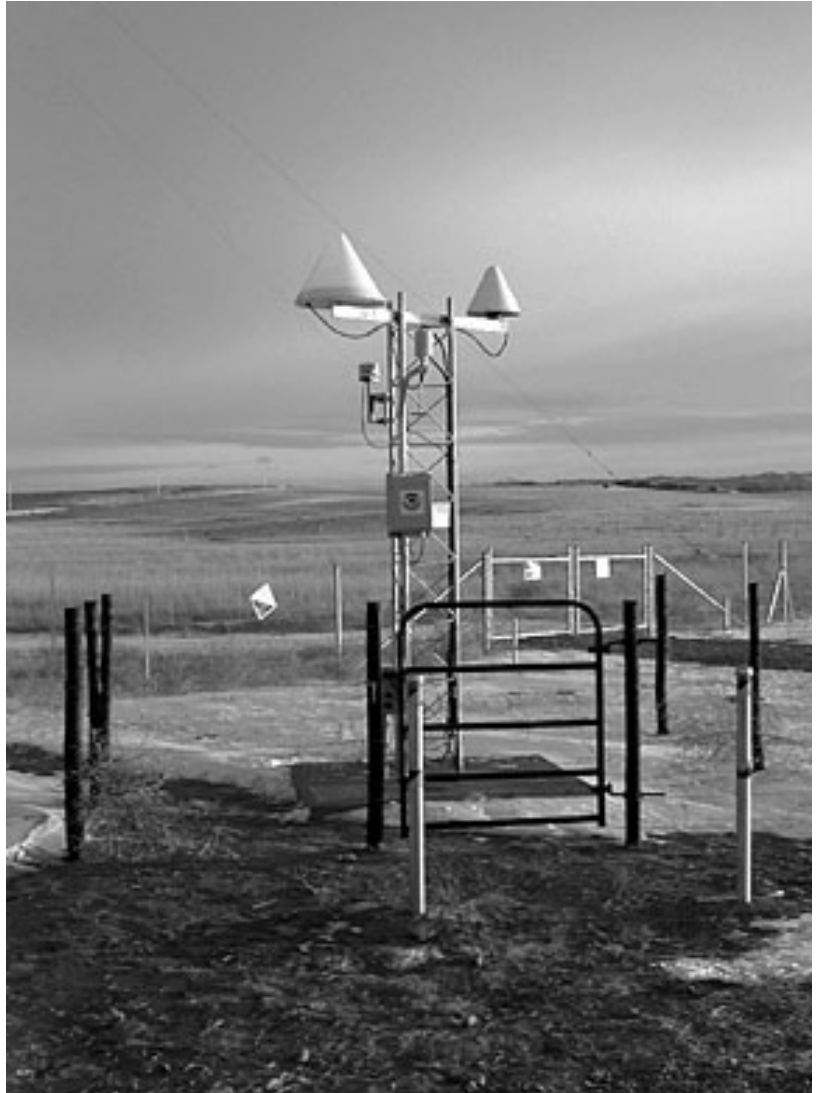
Figure 9. GPS-IPW installation at the DOT National Differential GPS site at Whitney, Nebraska.
