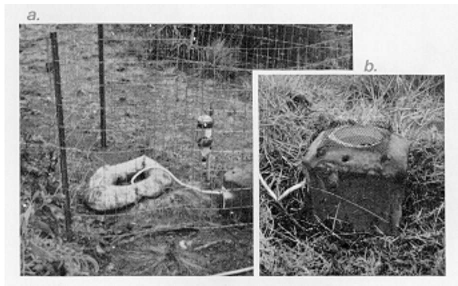
Figure 6. Constant-level pan evaporimeter. a) field installation with inner tube reservoir; b) evaporimeter detail. Note foam insulation around evaporation pan.
