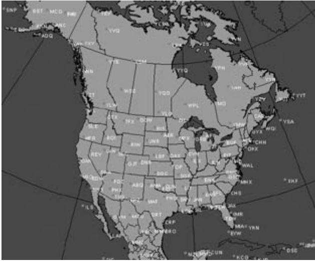
The North American network of upper air ground stations, each indicated by a three-letter station identifier. Radiosondes are launched and tracked from each location every twelve hours
