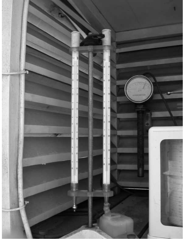
Figure 3. Psychrometer. Note the wet thermometer with its bulb covered by wet muslin (photograph courtesy of INM, Spain).
