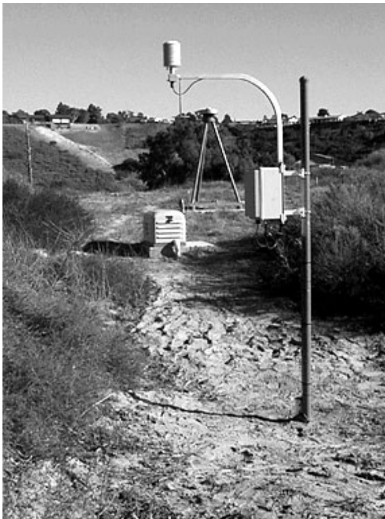
Figure 7. GPS-IPW installation at the Scripps Institution of Oceanography at La Jolla, California.
