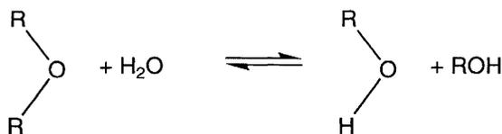
**Figure 4-37.** The hydrolysis of ethers.
