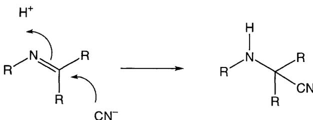
**Figure 4-29.** The formation of a cyanoamine by the addition of HCN to an imine.
