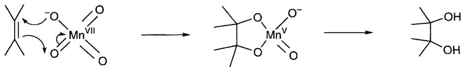
**Figure 9-34.** A likely mechanism for the oxidation of alkenes by high oxidation state oxo-complexes. The important feature is the formation and subsequent collapse of the cyclic ester.
