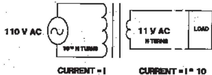
FIG. 3.4. Transformer uses two inductors to change 110 V of alternating current (AC) with current I (through 10 \cdot N turns) to 11 V of AC with current 10 \cdot I (through N turns). Note that power ( I \cdot V ) is conserved.
