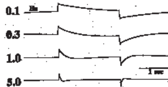
FIG. 3.10. Response of low-frequency filters to 50- \mu\text{V} square-wave calibration input, with respective cutoff frequencies of 0.1-, 0.3-, 1.0-, and 5.0-Hz.
