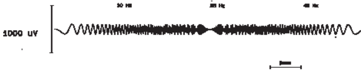
FIG. 9.15. Effect of aliasing caused by inadequate sampling rate. This sine wave recording sweeps through a frequency range of 0–50 Hz at a constant voltage and a sampling rate of 50 Hz. Notice the effect on the 25-Hz frequency.
