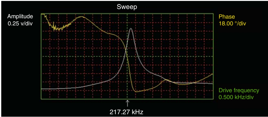
Fig. 2.21 Amplitude A (curve with maximum) and phase response of TM–AFM cantilever
