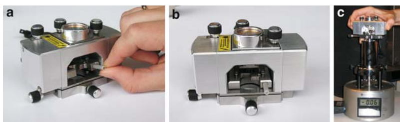
Fig. 2.6 (a) Insertion of cantilever holder; (b) premounted cantilever holder (the holder has been fixed by tightening the corresponding screws, compare Fig. 2.5d); (c) mounting of cantilever holder/optical head assembly onto the scanner
