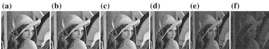
Fig. 5.5 Decryption results for a–c phase images and d–f amplitude images: multiplicative Gaussian noise with coeff. k = 0.2, 0.6, 1.8
