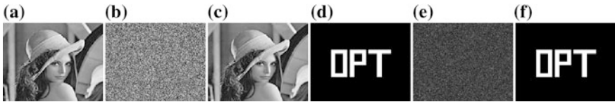
Fig. 5.3 a Input grayscale image, b encrypted image, c decrypted image and d–f corresponding results for binary image
