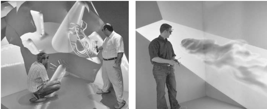
Fig. 4 Immersive investigation of fluid flow: Efficient depiction of particle trajectories via bill-boarding inside a blood pump (left) and volume rendering of temperature within a film cooling simulation (right)
