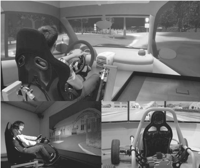
Fig. 11 Flexible presentation setup for VND: scaling VND from simple desktop-version to full-scale simulator application
