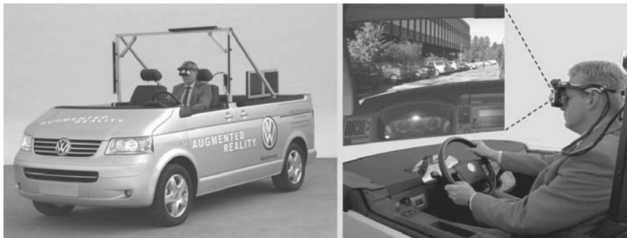
Fig. 15 Mobile AR test bench with tracking system for position detection (left) and virtual car components in driver's field of view (right)
