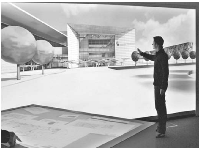
Fig. 2 HEyeWall 2.0 — tiled stereoscopic Virtual Reality display
