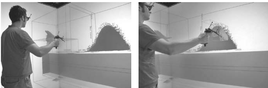
Fig. 3 A user interactively marks interesting value ranges in three-dimensional scatterplots. The combination of direct interaction and quantitative data display allows domain experts to control the feature extraction process
