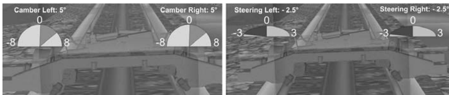
Fig. 34 Visualization of camber (left) and steering angles (right) of two wheels in the RailCab undercarriage
