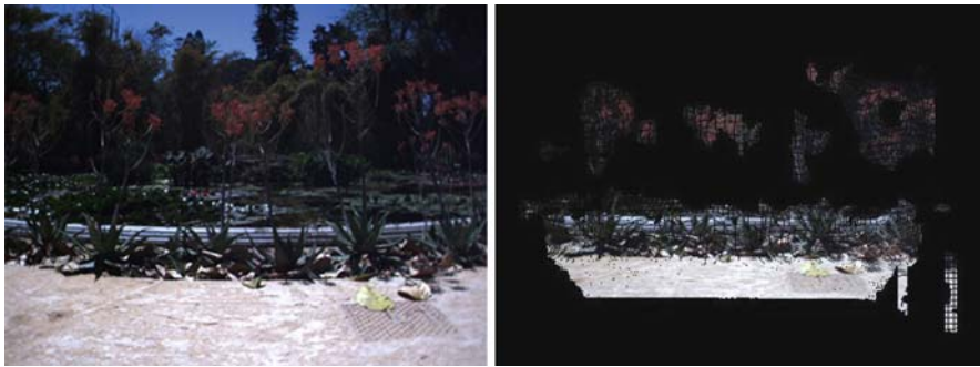
Fig. 10 Basin place ( left ) and its anticipation by the vision based perception loop ( right )
