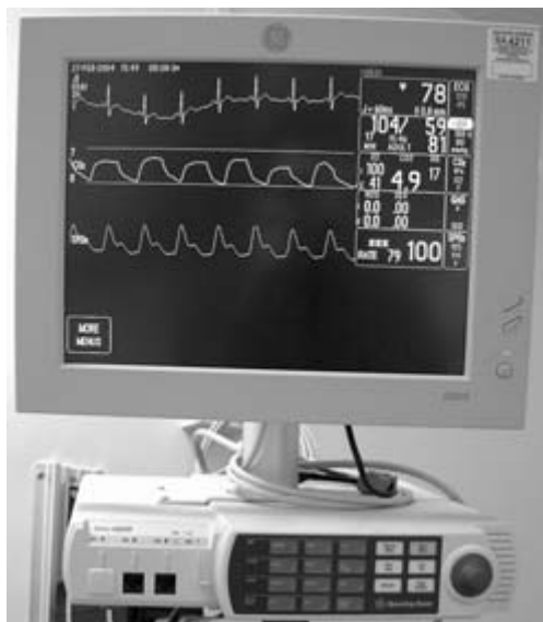
Figure 2.18 Integrated monitoring system displaying ECG and heart rate (beats/min), non-invasive blood pressure (mmHg), capnograph and end tidal carbon dioxide (kPa), pulse oximeter waveform and saturation (%).
