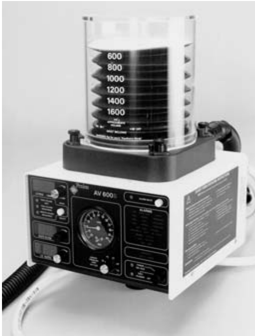
Figure 2.16 Photograph and diagram of bag-in-bottle ventilator. A, high-pressure driving gas input; B, anaesthetic gas output to patient.
